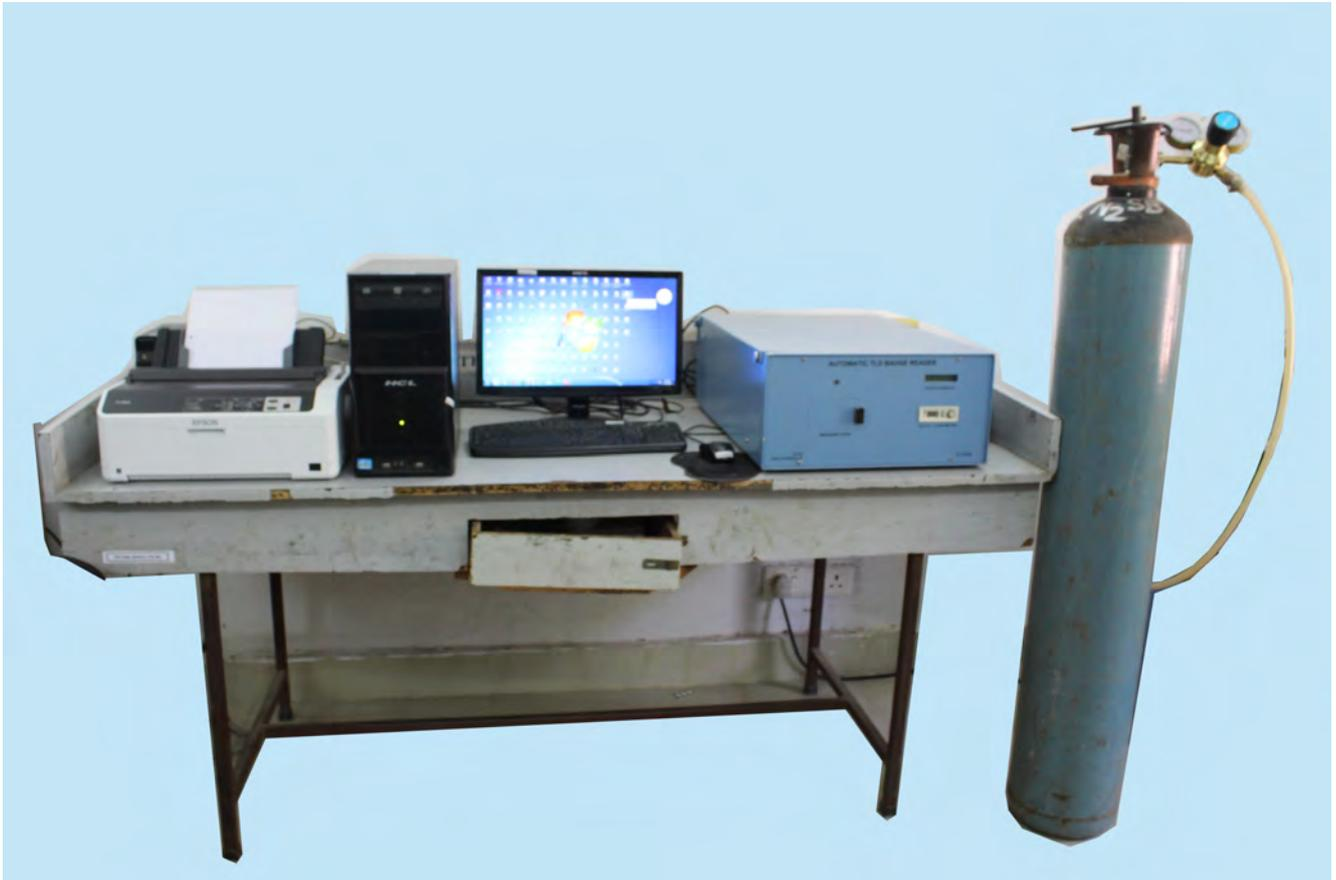
**Semi-auto TLD reader setup with PC & Nitrogen gas cylinder adjacent**
