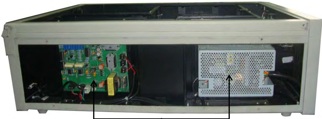
SMPS power supplies are in this design resulting in no use of bulky power transformers
